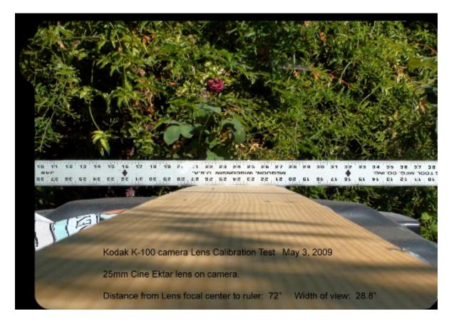
Lens Optical Center to Ruler: 72" Ruler angle to camera centered line of view: 90 degrees Ruler width: 48" Ruler visible in film frame: 28.8" total width (Horizontal view)
