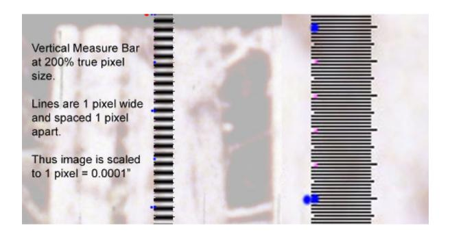
A second set of measure bars have also been developed, for angular measure across a horizontal field of view. This angular measure has three measure bars, one each for a 25mm lens, a 20mm lens, and a 15mm lens (using 22.62 degrees for the 25mm lens, based on lens tests, a 28.58 degree angle for the 20mm lens, based on calculation, and a 37.5 degree angle of view for the 15mm lens, based on calculation).
