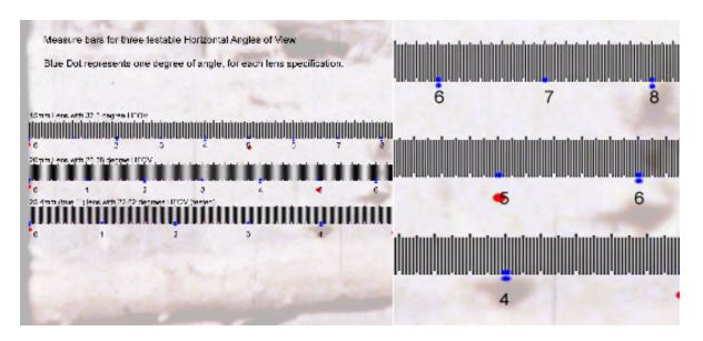
So using this set of three bars allows the tree or object elements in each test frame to be measured in angular position across the horizontal field of view, for the three test angles which will be first used in the preliminary analysis.
